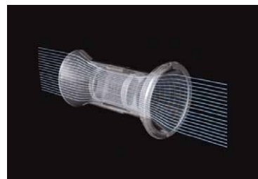
After – Turbulence has been significantly reduced in the bookshelf speakers' CFD-designed ports
