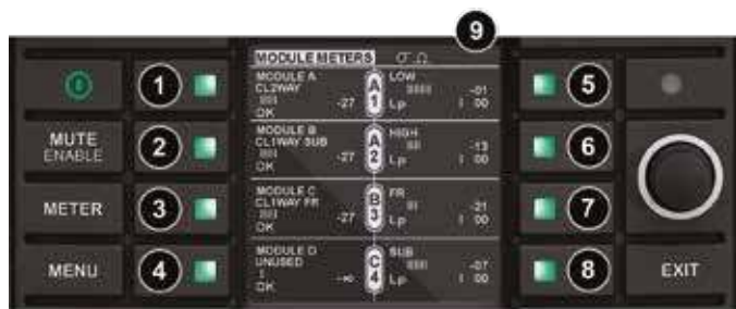
Figure 7.12: Meter Mode > Module Meters View
