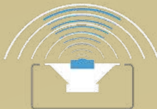
Wide dispersion of mid frequencies, narrow dispersion of high frequencies
