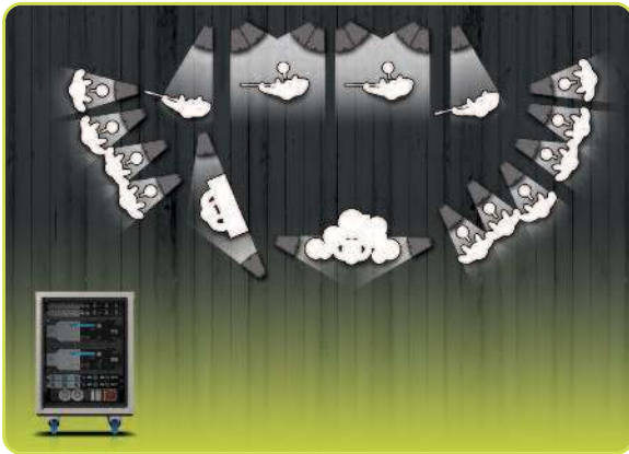
24 x 45°N12 monitors powered by a single NUAR rack.
