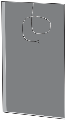
Fig. 3. Drywall Cutout with Speaker Cable
